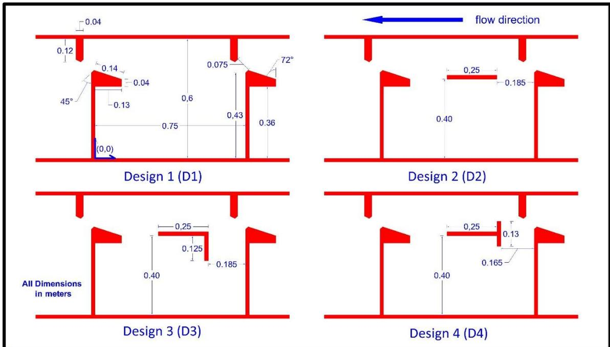
Fig. 7 Diagrams of the standard design and the modified designs
