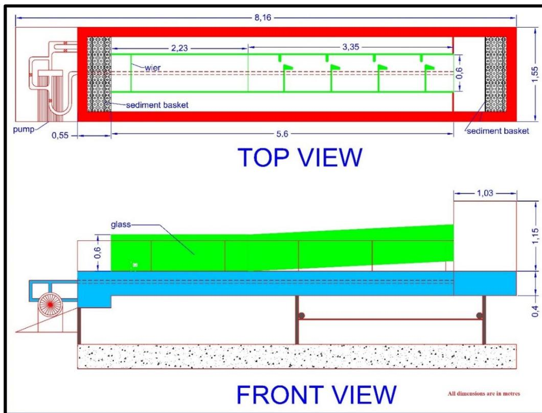
Fig. 4 Schematic of the laboratory channel
