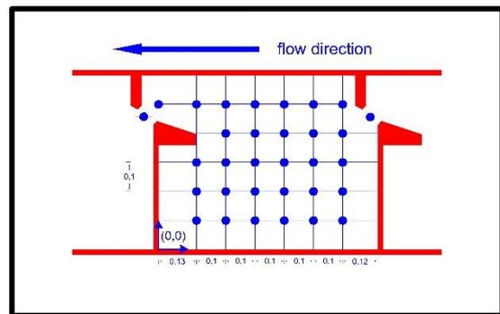
Fig. 6 Illustrates the mesh points for velocity readings, all dimensions in meters
