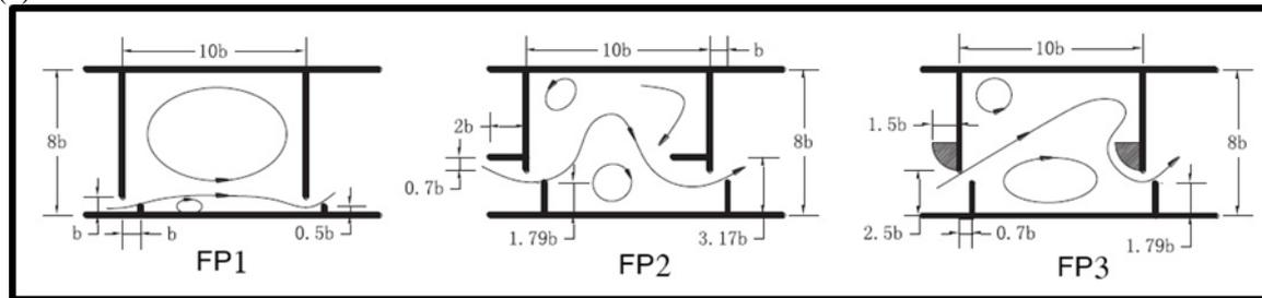
Fig. 2 Illustrate of flow patterns in one chamber [24]
