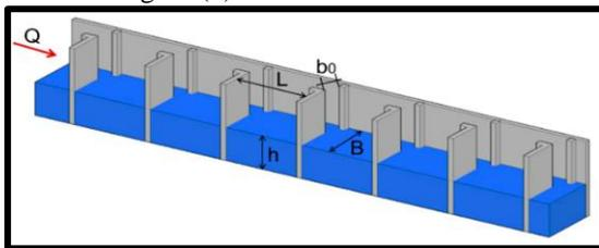
Fig. 1 Schematic of Vertical Slot Fishway [14]
