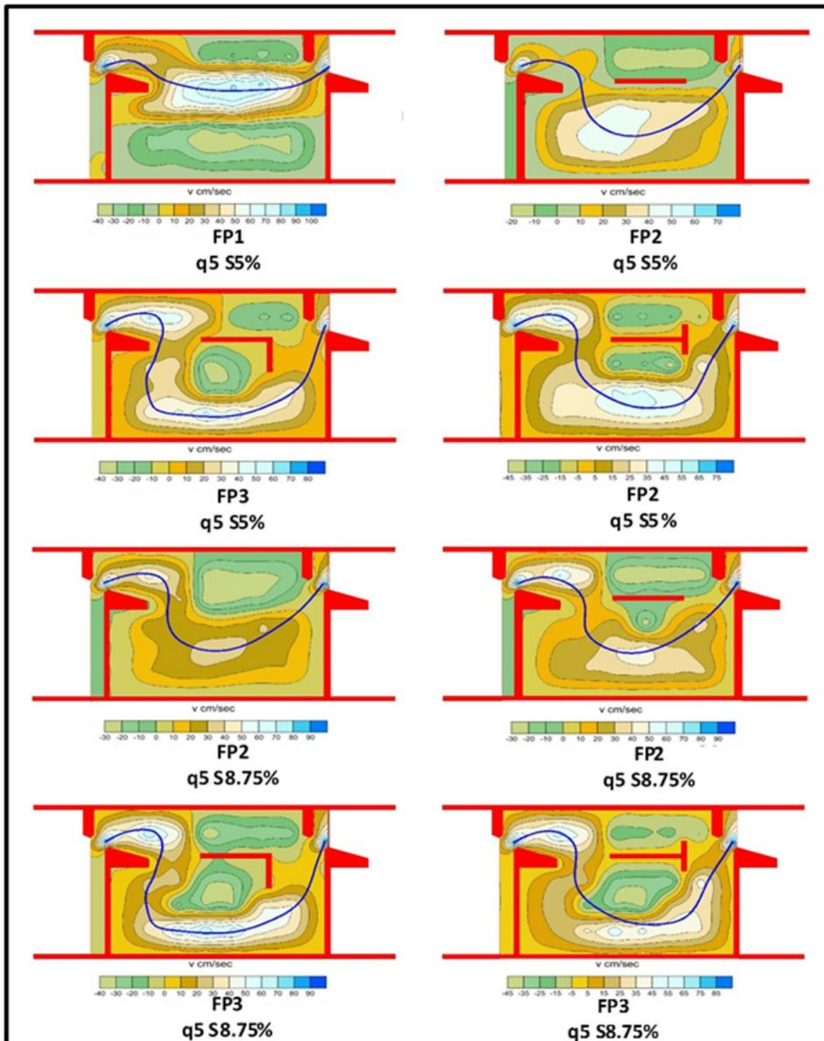
Fig. 9 Illustrates the effect of the modifications inside the basin on the flow pattern for the case of discharge  $q_5$  and slopes 5% and 8.75%.
