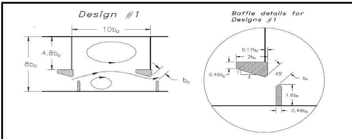
Fig. 5 schematics of the standard vertical slot fish pass according to [33].
