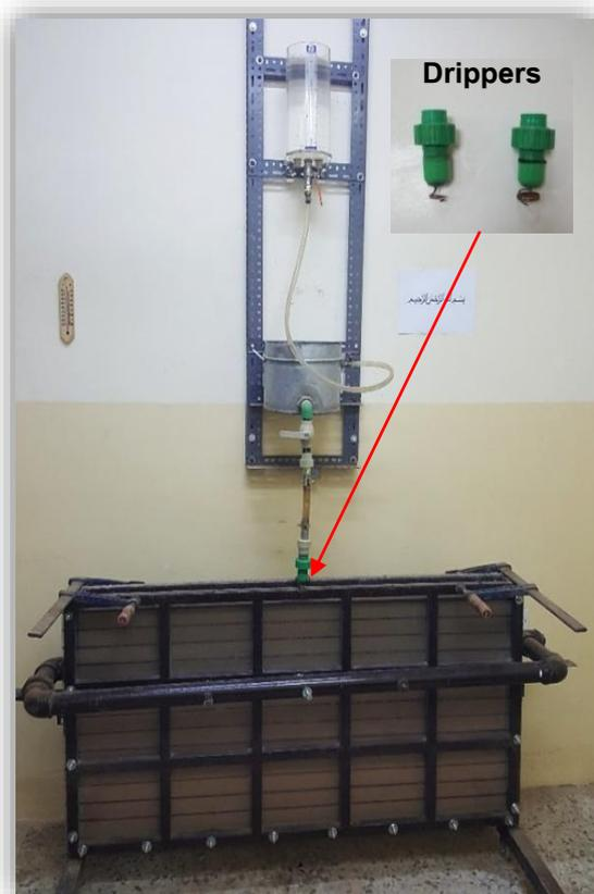
Figure (1): Laboratory soil container and water preparation system
