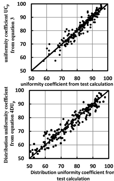
Figure (12): Uniformity coefficient and distribution uniformity coefficient Values calculated from the tests and from equations 3 & 4.
