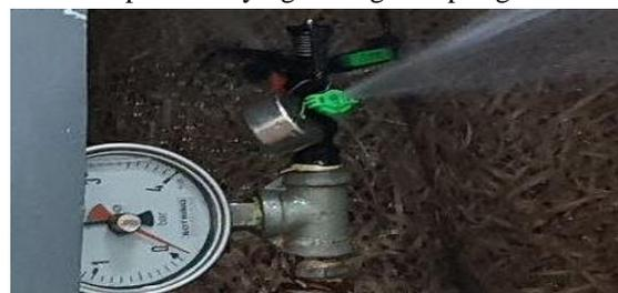
Figure (7): Slowing down the rotation of the sprinkler by adding weight to the impact arm.
