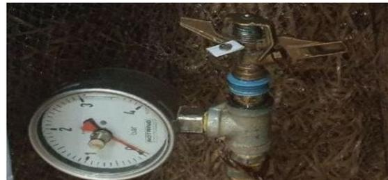
Figure (6): Accelerating the rotation of the sprinkler by tightening the spring.
