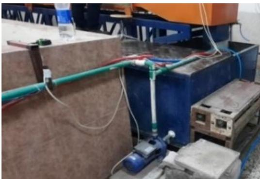
Figure (5): Water supply tank and main pump.
