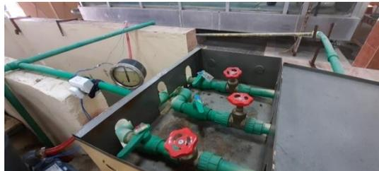
Figure (4): Valve control box for pressure head change.
