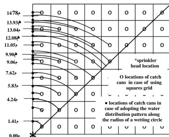
Figure (1): Water distribution pattern of a single sprinkler resulting along the radius of a wetting circle centered by the sprinkler head.
