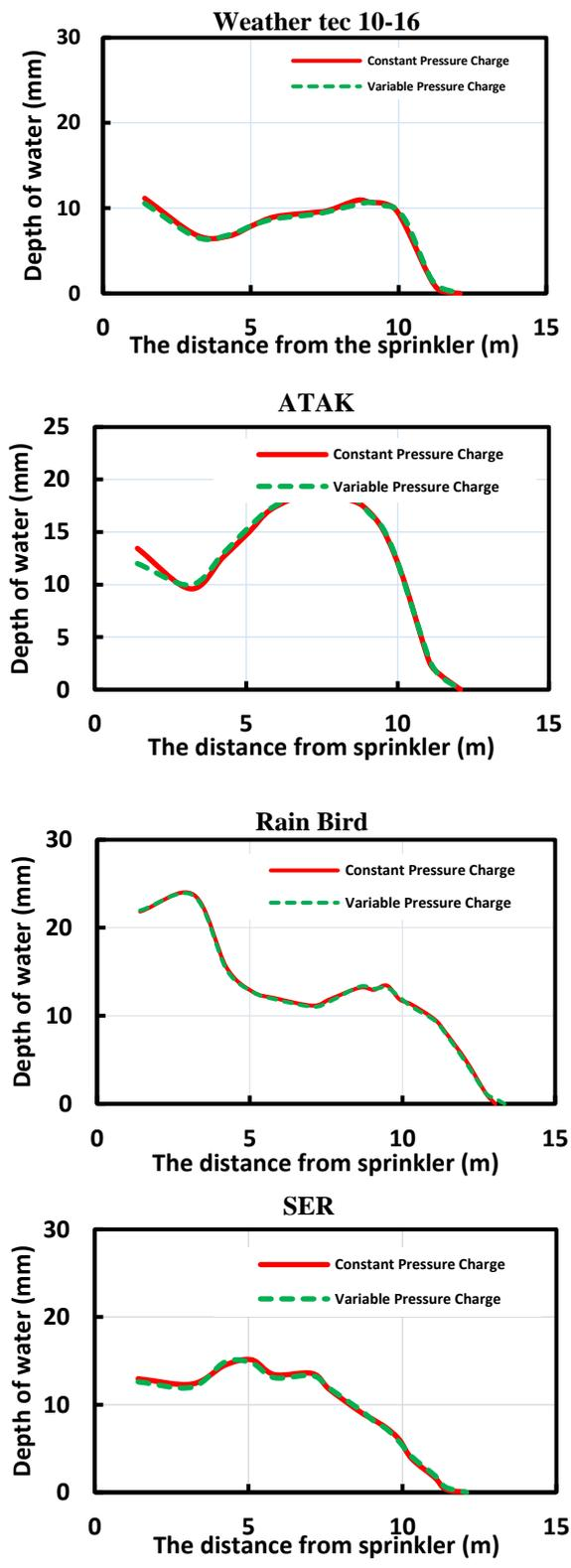
Figure (10): Water distribution pattern for a single sprinkler under constant pressure head and variable pressure head and for all sprinkler heads in this research.
