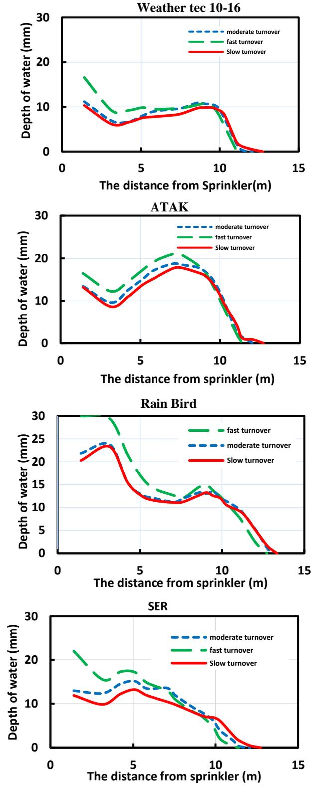
Figure (11): Water distribution pattern for a single sprinkler under constant pressure head and for different cases of sprinkler rotation speed and for all sprinkler heads in this research.
