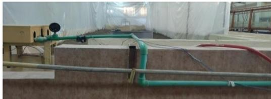
Figure (3): Supply pipe, pressure control, water return pipe, and excess water return pipe.
