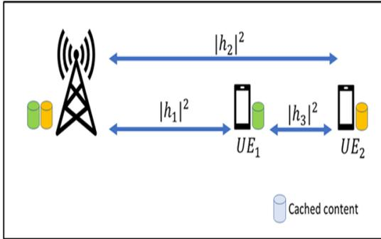
Fig. 2 The System model for C-NOMA with caching
