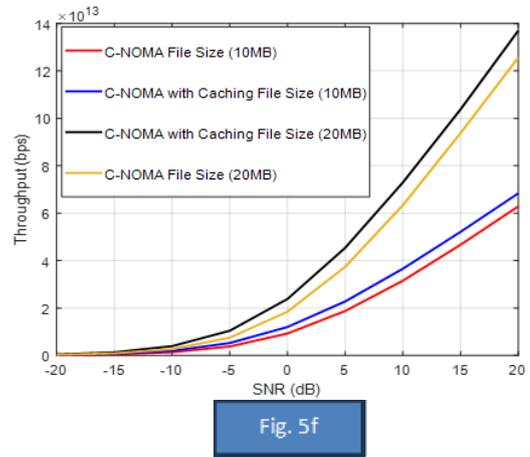
Fig. 5 Throughput comparison between the C-NOMA with caching versus traditional C-NOMA for different cases
