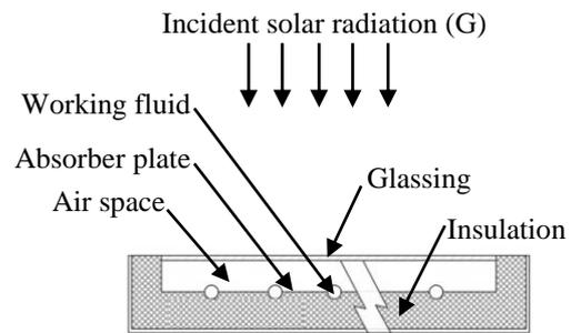
Fig. 1 Schematic diagram of flat-plate solar collector
