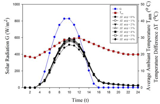
Fig. 6 Variation of hourly solar radiation on the solar collectors, ambient temperature and working fluid temperature differences as a function of nanoparticle volume fraction during a typical day in October.
