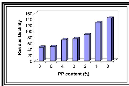
Fig. (2) Relationship between Polypropylene content and Residue
