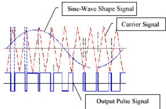
**Fig. 3 PWM Signal Synthesis**
