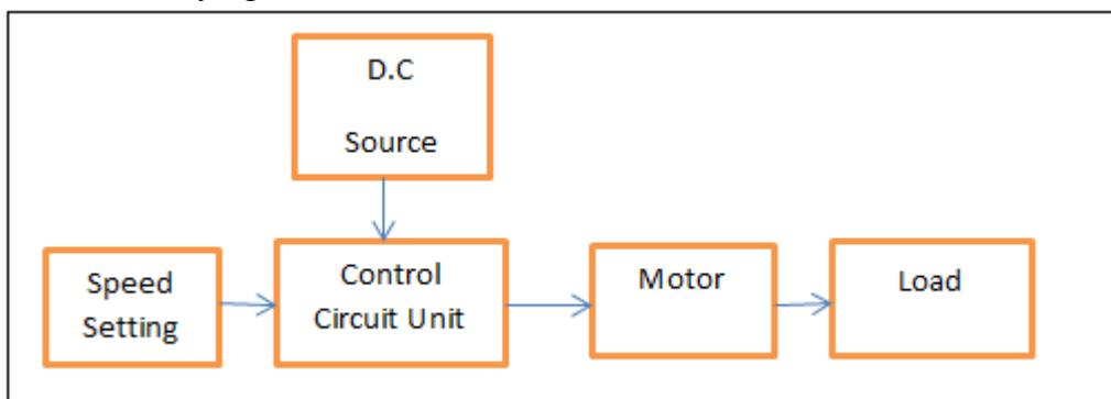
Fig. 4 Block diagram of open-loop control
