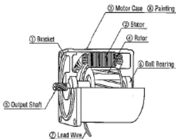
Fig. (1) Construction of the single-phase induction motors
