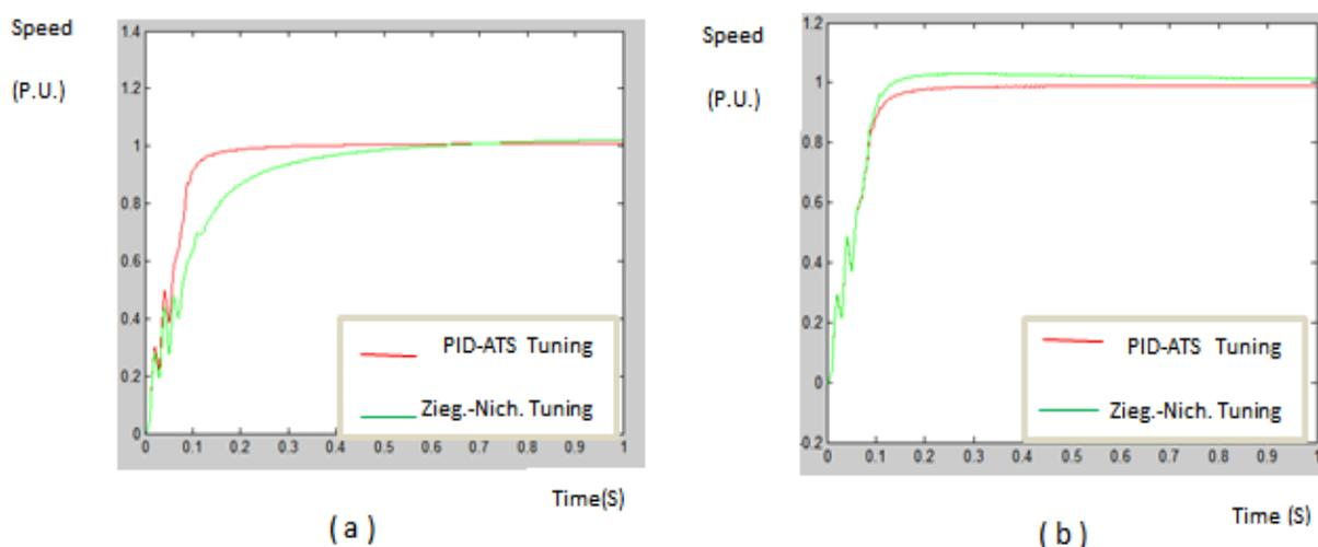
**Fig. (12) Comparing performance of PID-ATS controller and Ziegler-Nichols Controllers at**
